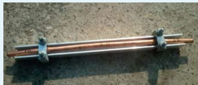
Fig. 3 : Copper tube for noble gas sampling
